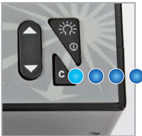
Press and HOLD the 'C' key to start calibration.
